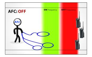
Although AFC helps radios to continue to communicate, it can only temporarily correct a certain amount of oscillator drift; 1000 Hz or 1500 Hz depending on the manufacturer. A low battery will also abruptly disengage AFC. Once the drift exceeds a certain threshold value, the embedded process will no longer attempt to correct the problem, thereby resulting in a hard failure.
